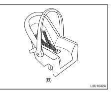
A rear-facing infant seat (B) provides restraint with the seating surface against the back of the infant. The harness system holds the infant in place and, in a crash, acts to keep the infant positioned in the restraint. A forward-facing child seat (C-E) provides restraint for the child's body with the harness and also sometimes with surfaces such as T-shaped or shelf-like shields.
